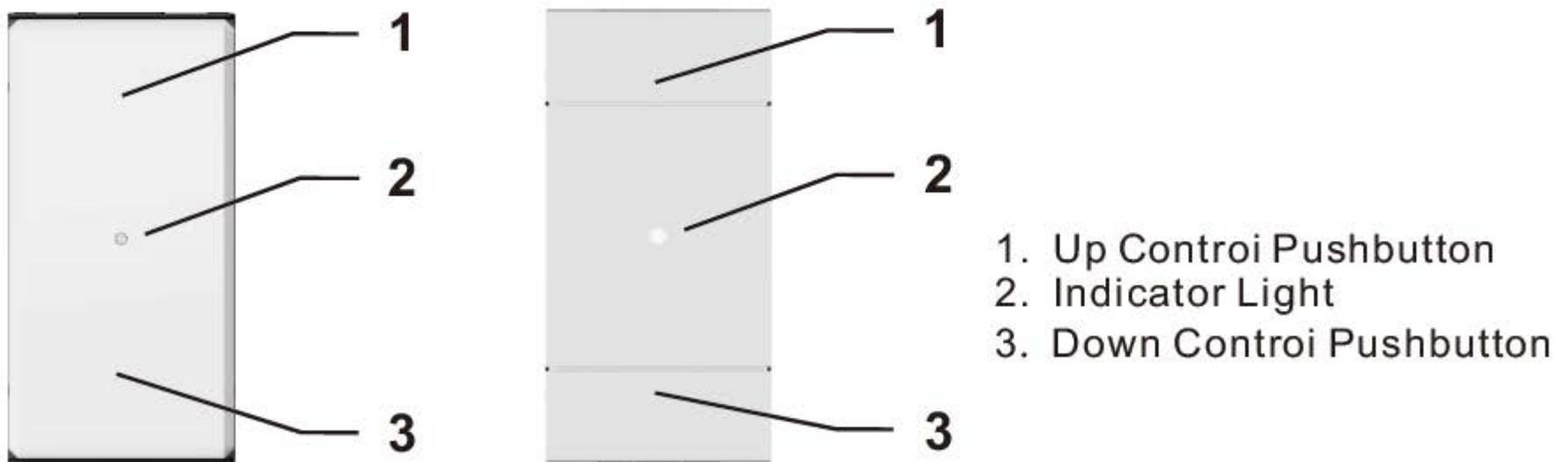
⚠ The device will exit Pairing Mode if not paired within 3 minutes. To re-enter this mode, press and hold the 'Up' and 'Down' control pushbuttons simultaneously for 5 seconds. The blue indicator light will flash, and the device will enter Re-Distribution Network Mode.
